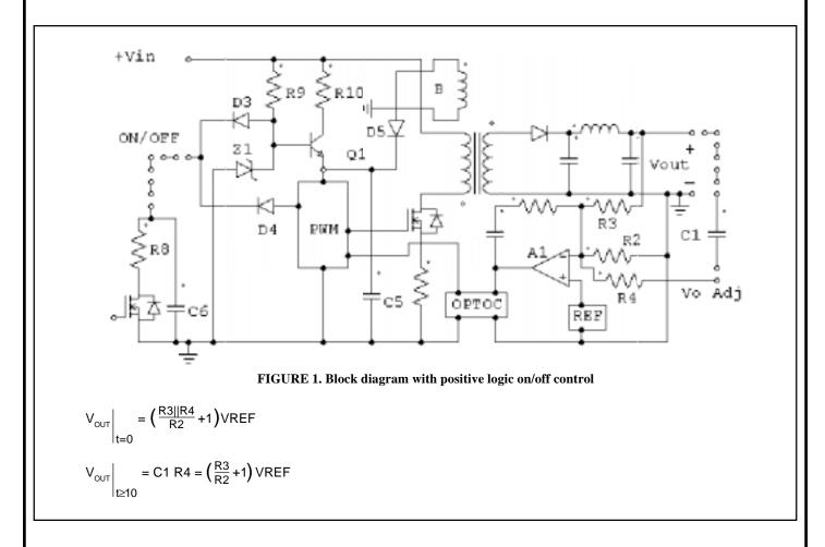
Figure 1 shows the block diagram of a flyback converter with the bias circuitry for the control IC (PWM) and the feedback loop consistent of the error OPAM A1 and the optocoupler. When Vin is applied while the on/off pin is open, the zener diode Z1, which is biased through R9, holds the base of Q1 at  $V_z$ . The emitter voltage of Q1 biases the PWM until the output Vout reaches its steady state and is then forced off by the voltage
