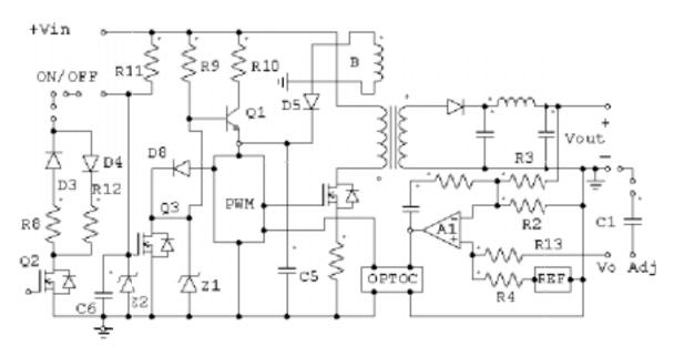
FIGURE 3. Block diagram with negative logic on/off control
