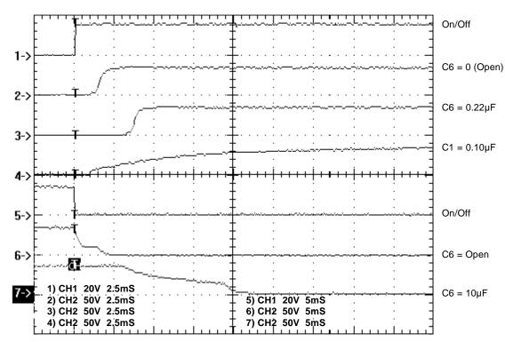
FIGURE 2. Turn on/off delay and soft start waveforms for the DC/DC converter in Figure 1
