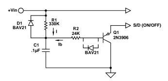
DELAY  $\approx 2.5$ mS/0.1µF for V<sub>IN</sub> = 12V FIGURE 2. Turn on delay circuit
