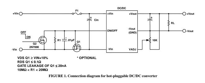
NOTE: The power dissipated by Q1 is given as:
