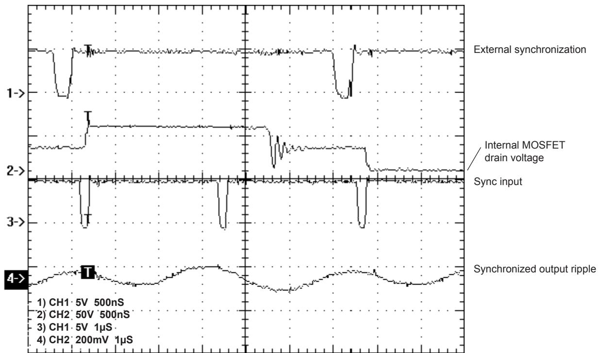
FIGURE 5. Synchronization waveforms
