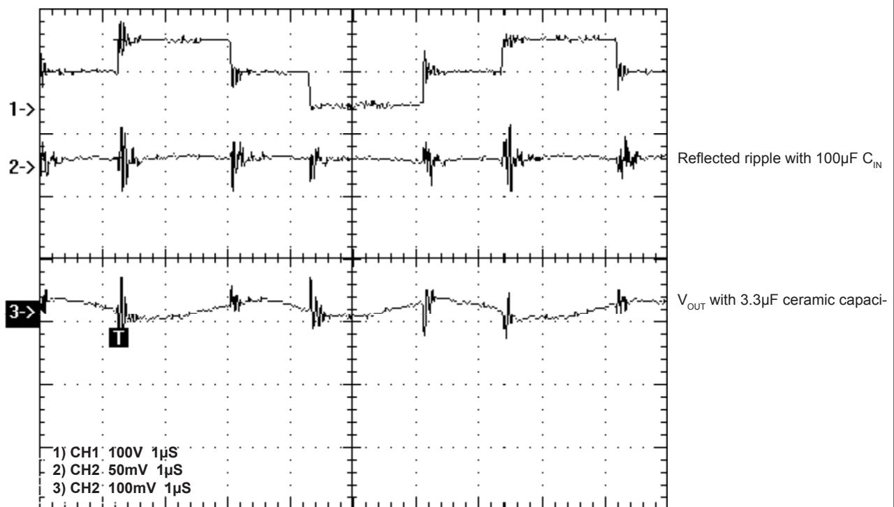
FIGURE 3. Reflected ripple and  $V_{\text{OUT}}$
