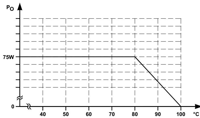
FIGURE 2. Typical derating curve with free air cooling
