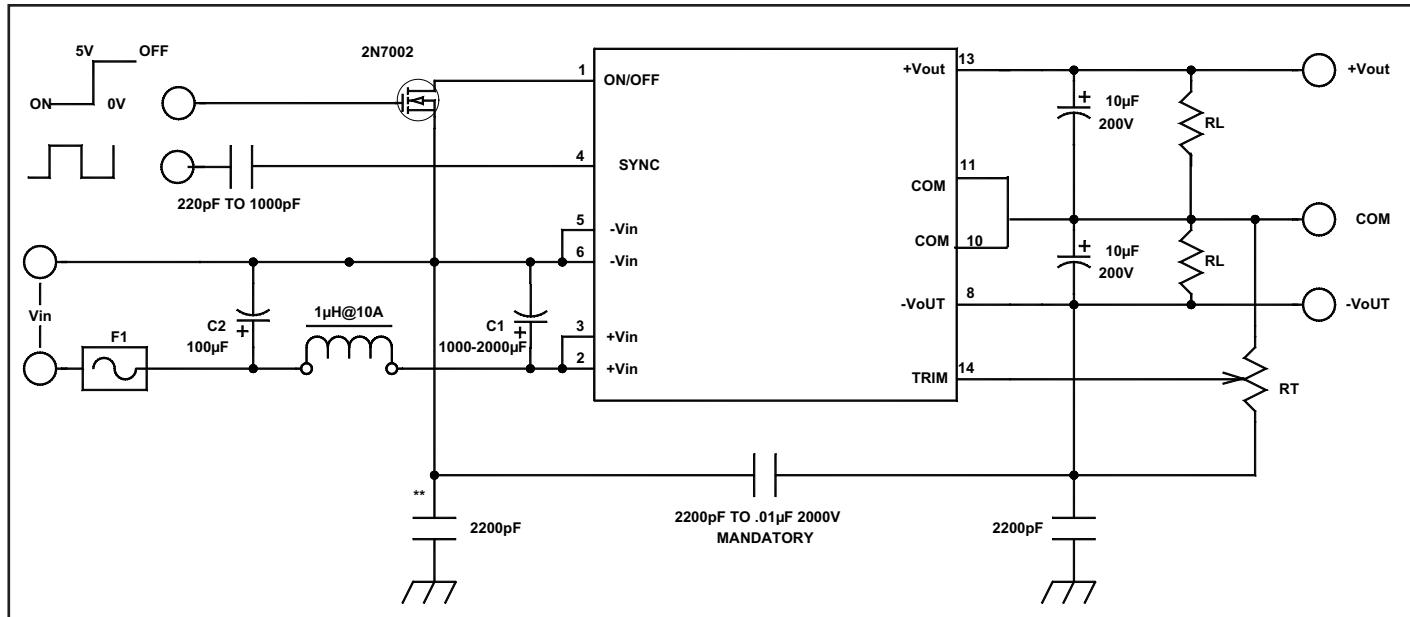
FIGURE 1. Typical connection diagram of BD15001 converter
