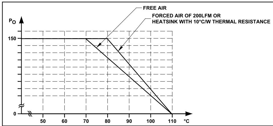
FIGURE 2. Typical derating curve with free air cooling
