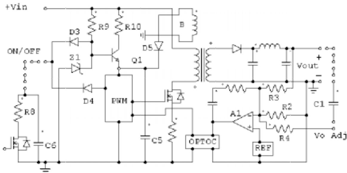
FIGURE 1. Block diagram with positive logic on/off control
