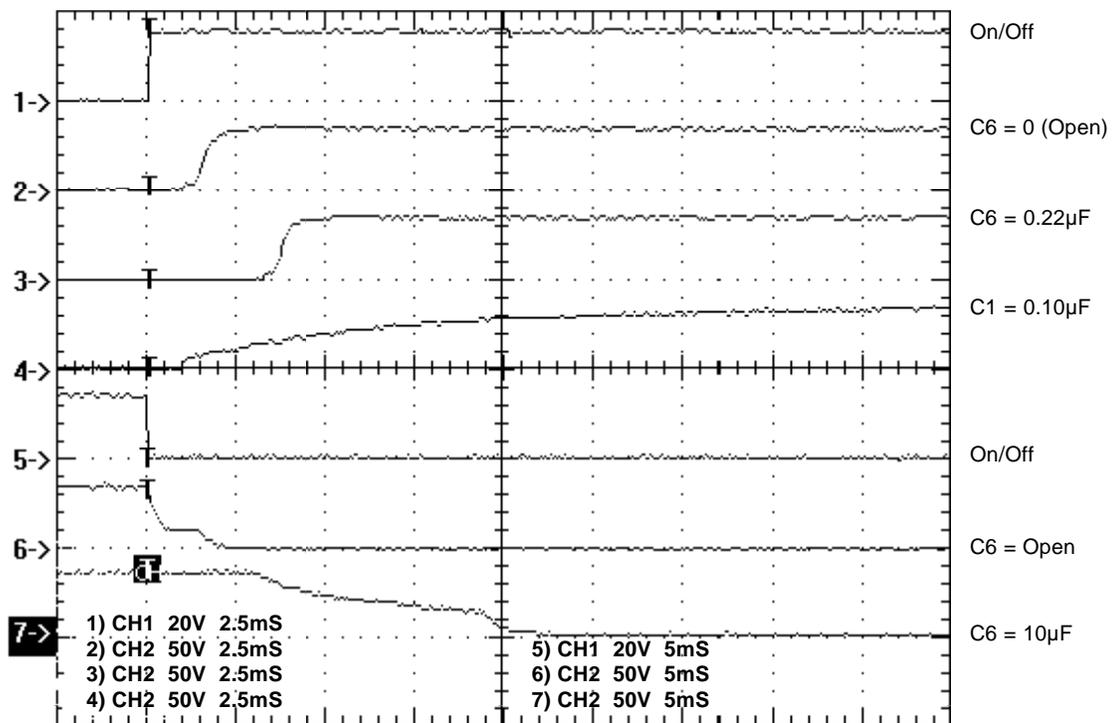
FIGURE 2. Turn on/off delay and soft start waveforms for the DC/DC converter in Figure 1
