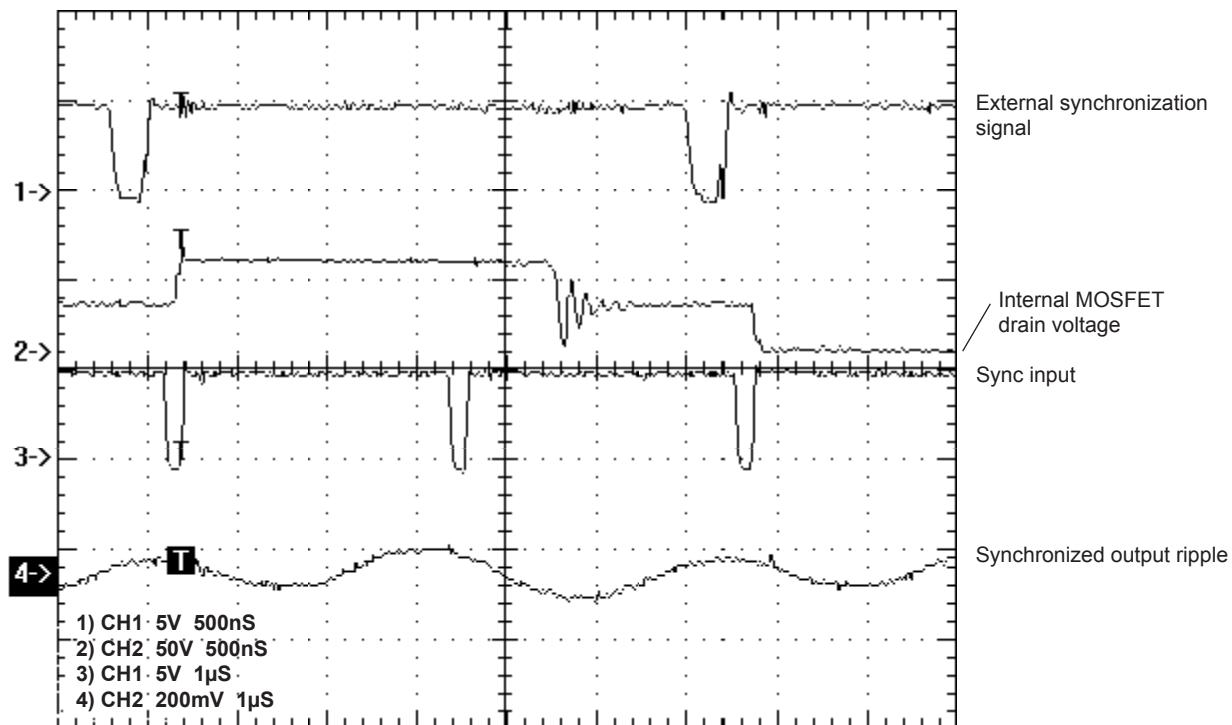
FIGURE 4. Synchronization waveforms
