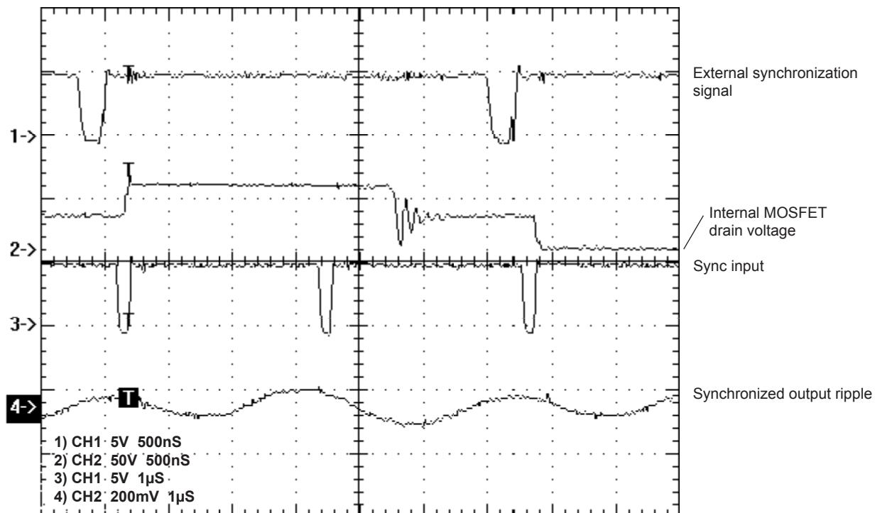
FIGURE 5. Synchronization waveforms
