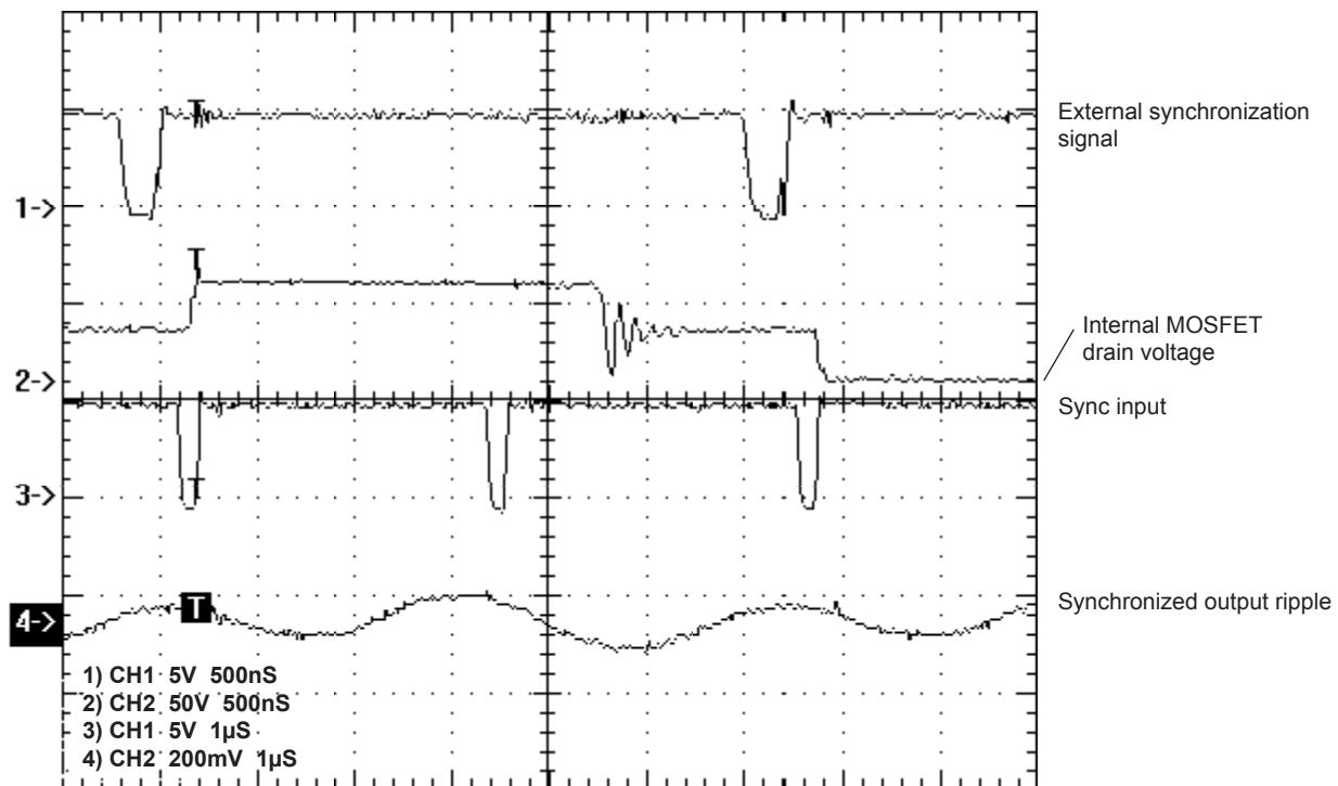
FIGURE 5. Synchronization waveforms
