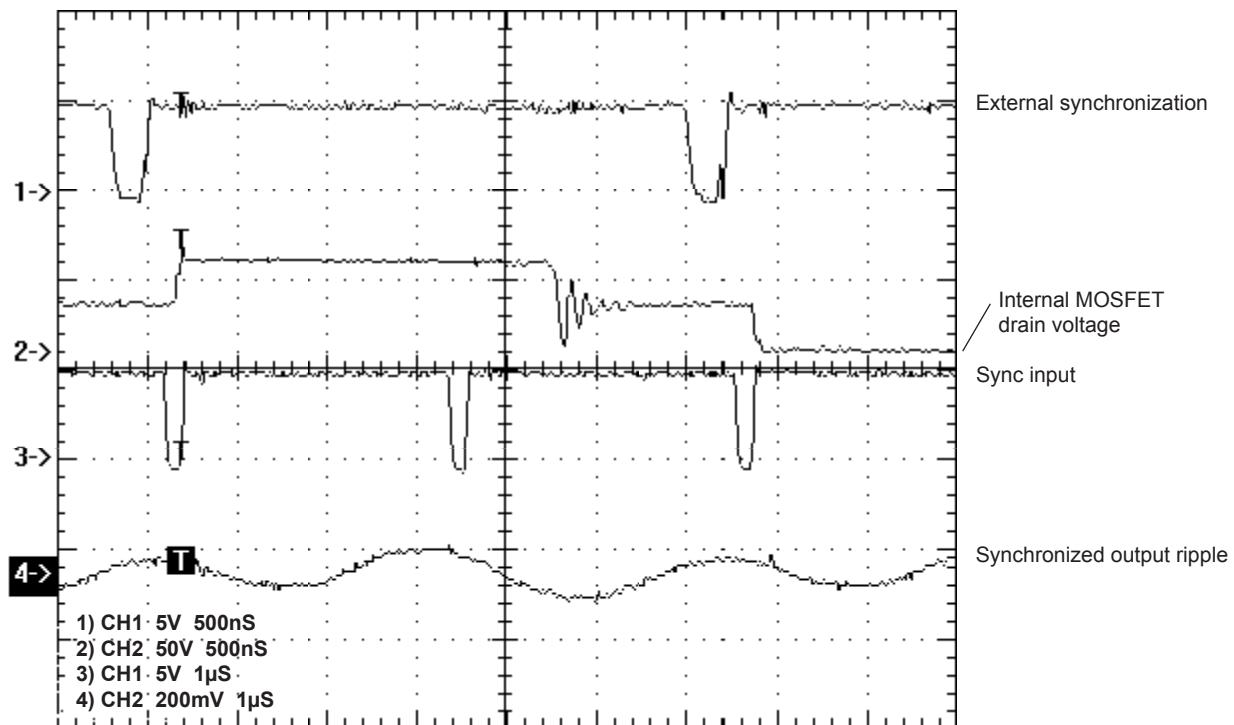
FIGURE 4. Synchronization waveforms
